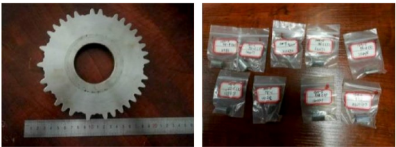
图 6 弯曲失效齿轮 Fig.6 Bending failure gear
